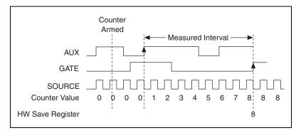
Figure 7-20. Single Two-Signal Edge-Separation Measurement
